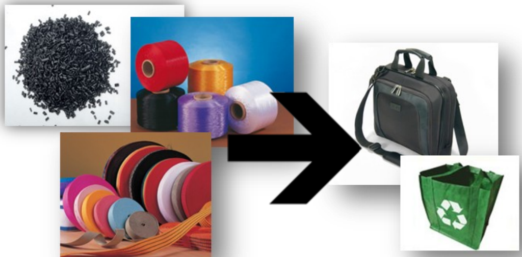
Fibre-grade recycled polypropylene pellets, Polypropylene filament yarn & Polypropylene consumer webbing products are recycled to manufacture consumer goods, such as belts and fabric for bags
